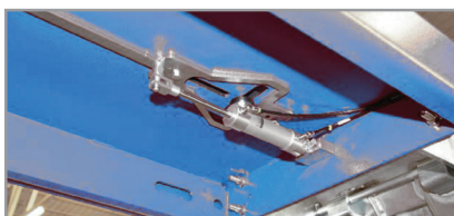
Central pneumatic locking of the sliding plate
