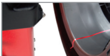
Lazer Indicator Precise positioning of the adhesive weights at 6 o'clock mark.
